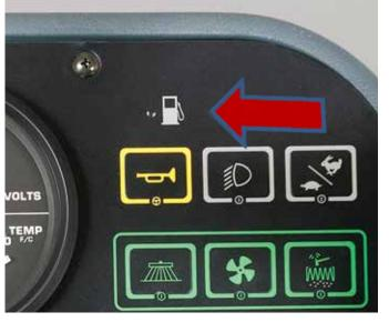
1. Check the diesel fuel tank level/LPG bottle/ Battery charge. In case refill/ change the LPG bottle.
