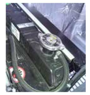
5. Check the engine liquid coolant level.
