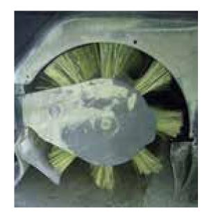
3. Check the main broom bristles wear out and Check that the main broom freely rotate and free from ropes or debris.
